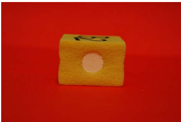
Fig. 3 Photograph of an augmentation model (cement used: Zn-GPC B) after 1 million load cycles in the compression fatigue life test
